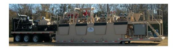
6,270+ gal 3 Section Tank 1000+ gpm Cleaning Capacity
